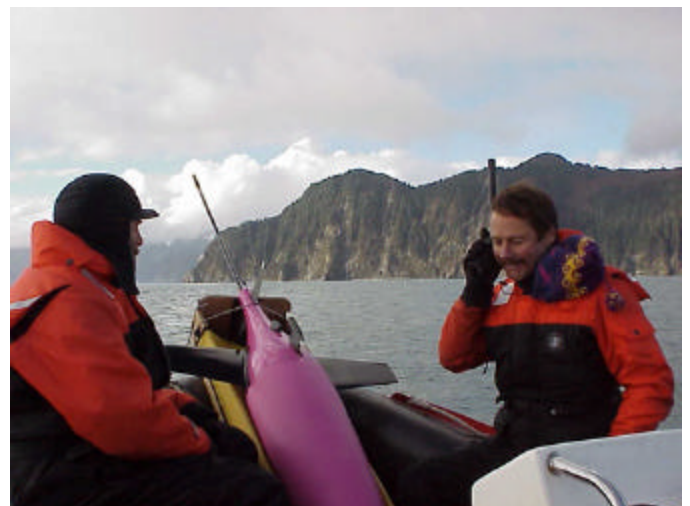
Figure 1. Jim Osse prepares Seaglider for launch from the University of Alaska - Seward Marine Center's inflatable boat. Seagliders can be easily manipulated by two people and are typically launched from small, flexible platforms such as inflatables and work boats. (Photo courtesy of Tom Lehman and Jim Osse.)
